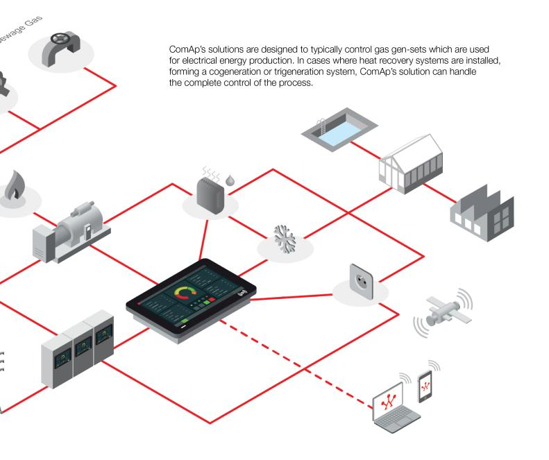
Our system controls the essential parts of the gas engine (e.g. Air/Fuel ratio to secure safe and reliable operation and emissions compliance), ensures compliance to local standards norms and requirements (e.g. grid connection rules - Grid codes) and interface to other on-site products such as ignition and others. Detailed system diagnostics are available both locally and remotely to make sure your system is available and running smoothly.
